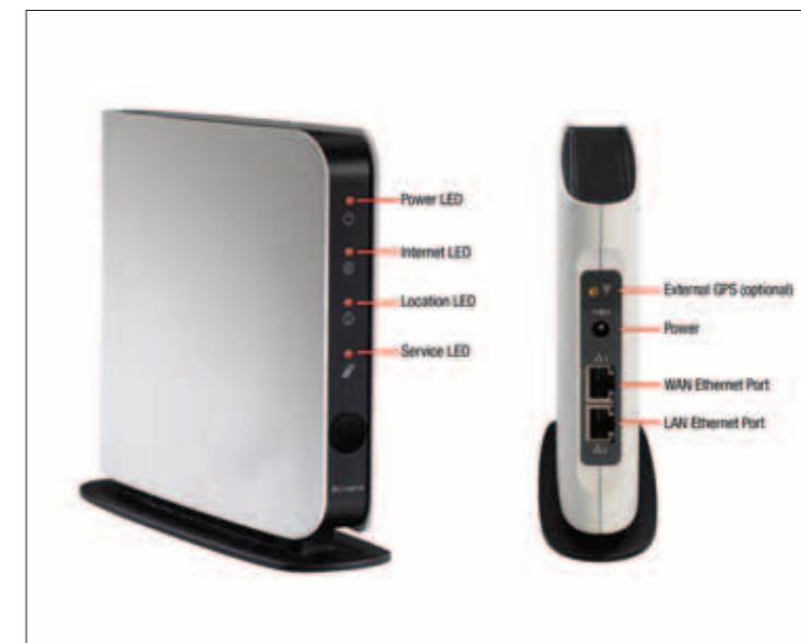
Femtocells can work efficiently across a much broader range of the radio spectrum than macrocell based systems. Airvana's HubBub UMTS femtocell is a hand-sized device that can deliver a throughput of data at 5 Mbps or quicker.
